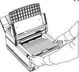
3. Remove the old image drum unit (with its toner cartridge), wrap it in the packaging materials from your new image drum unit and dispose of it following local regulations.
